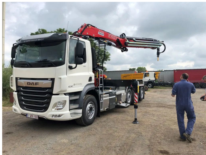
DAF CF 480 FAQ +Fassi Kraan F235A2.24 + Container... 8x2
